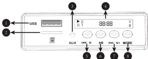
Auto-Play function is enabled when an external USB / TF card media controller detected.
