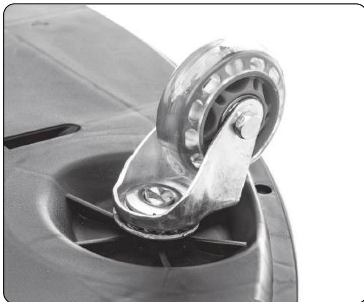
1. Install front wheels by firmly pushing down into the main body.
