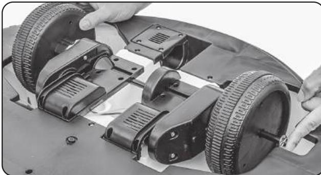
3. Slide axle to either side to properly insert rear wheel. Ensure the wheels are aligned with sprocket.
